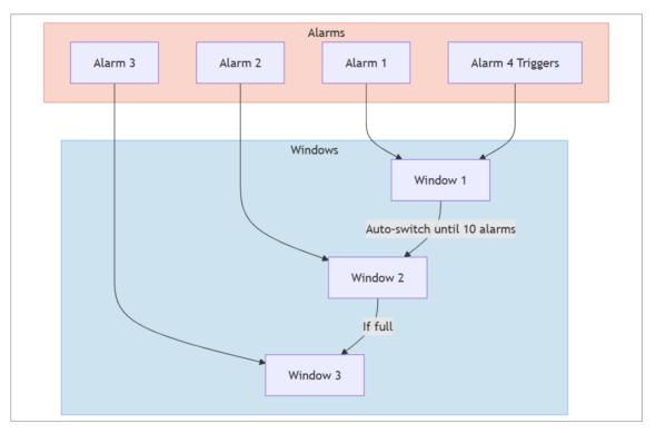
Figure 14-25 Multiple Alarm Windows Under Auto-Switch Mode
