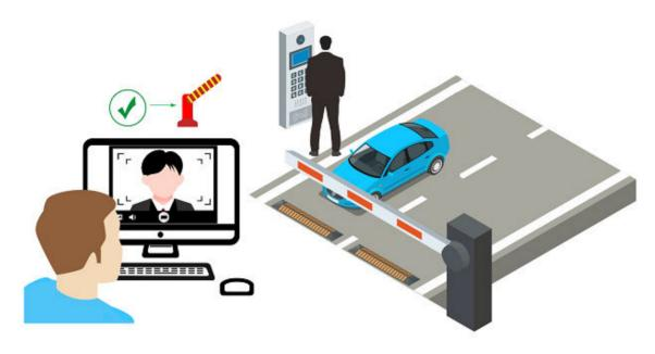
Figure 11-6 Start Video Intercom to Send Opening Barrier Request
