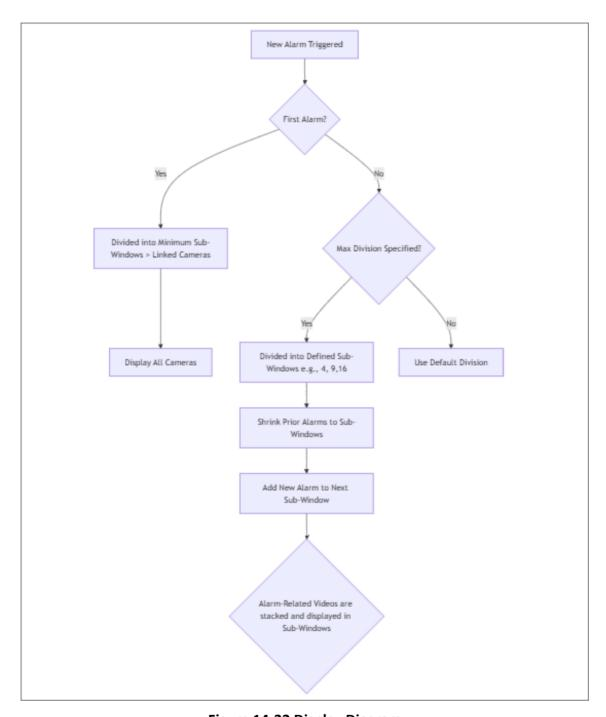
Figure 14-22 Display Diagram
