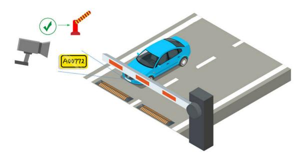
Figure 11-2 Example: Barrier Opened Automatically for Vehicle in Vehicle List
