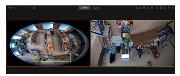
Figure 4-8 Dewarped Zooming Area Window (Fisheye Camera)
