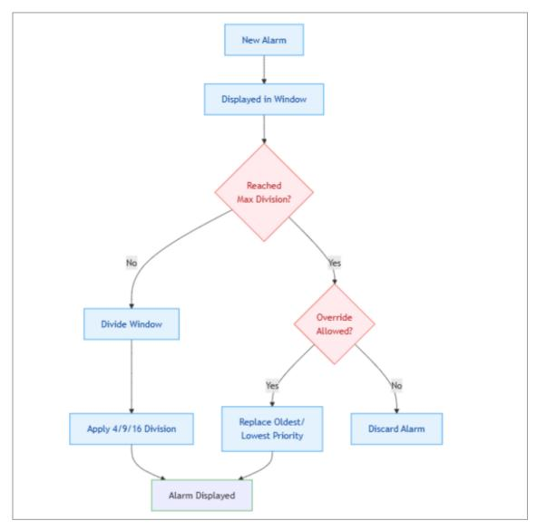
Figure 14-19 Display Diagram
