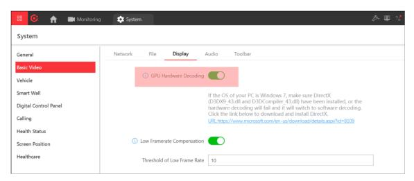
Figure 14-30 Enable GPU Hardware Decoding
