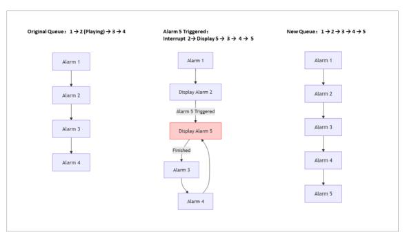
Figure 14-24 Single Alarm Window Under Auto-Switch Mode
