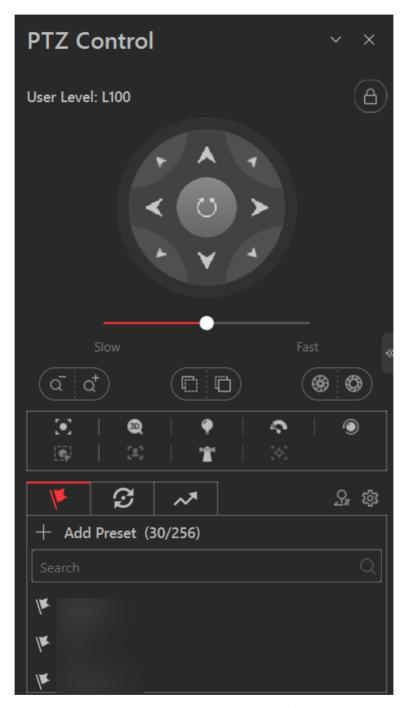
**Figure 4-1 PTZ Control Panel**
